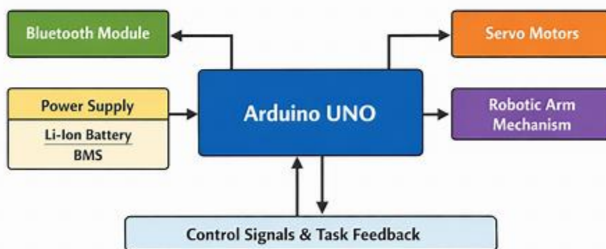
Figure 5: Block diagram of the Arduino-based 5-DoF robotic arm system
